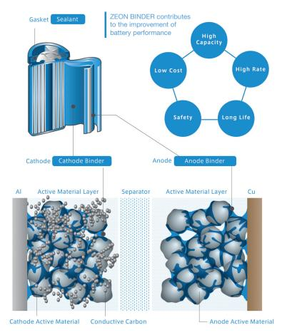
ZEON will be demonstrating its line of aqueous and NMP-based binders for Li-ion anodes and cathodes at AABC 2014. These binders provide improved electrochemical performance, require less amount of binder, and offer reduced overall cost as compared to cells made using PVdF. In the exhibition hall, ZEON will introduce its latest advancements for cathode binders and both water-based ceramic and polymer particle functional layer coatings.
